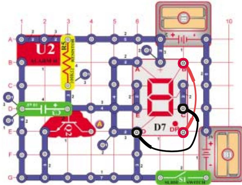
The circuit switches between numbers "3" and "6" on the display. Place a jumper from segment C to segment D and segment B to segment DP.
