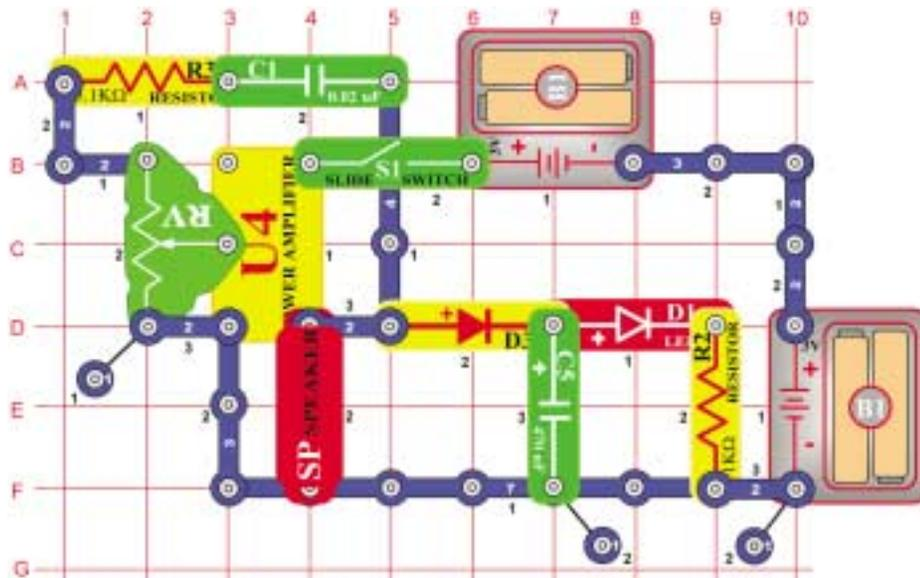
This circuit is based on the Trombone project #238. Turn on the switch (S1) and set the variable resistor (RV) for mid-range for the best sound. The LED (D1) will also be lit.
