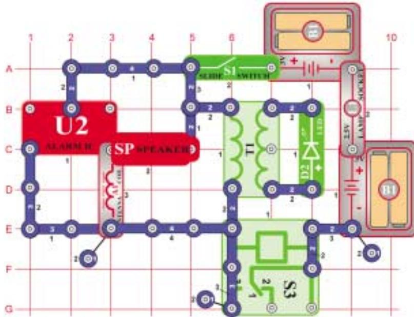
Turn the switch (S1) on and the speaker (SP) sounds as the motor (M1) spins. The relay's (S3) contacts rapidly open and close the battery connection to the circuit causing the alarm IC (U2) sound to be different.
