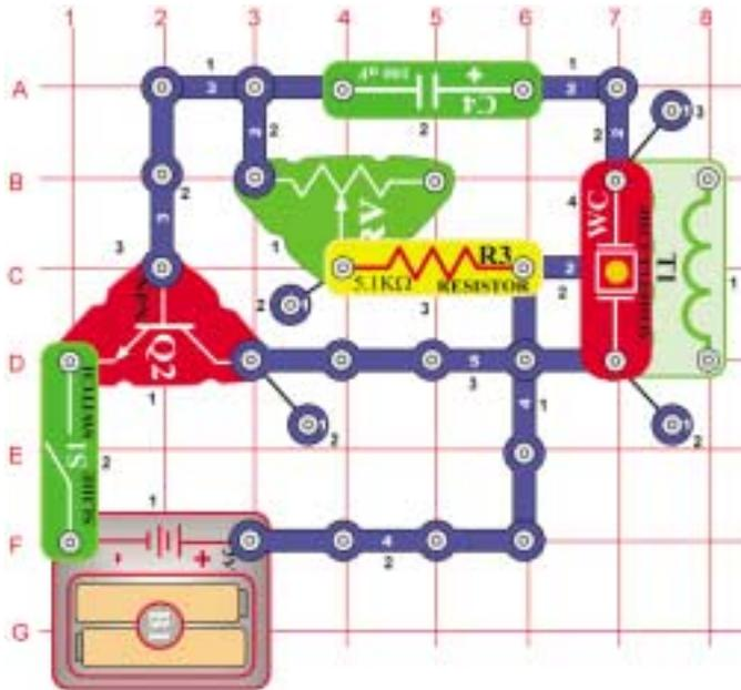
Build the circuit and set the variable resistor (RV) control all the way to the right. Turn on the switch (S1) and you hear a sound like a faucet dripping. You can speed up the dripping by moving the variable resistor control around.
