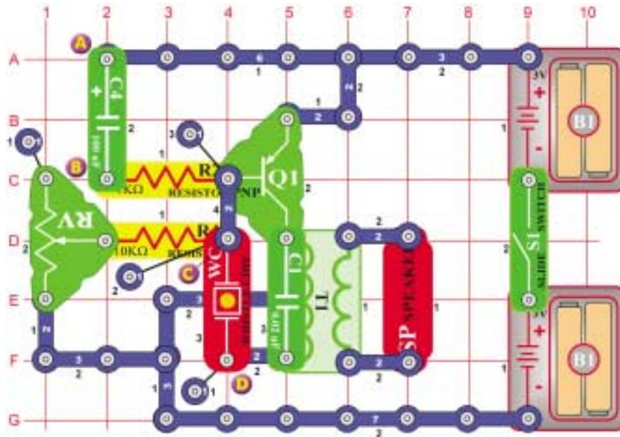
Turn the switch (S1) on and this simple oscillator circuit outputs a beep from the speaker (SP). Change the frequency by adjusting the variable resistor (RV).
