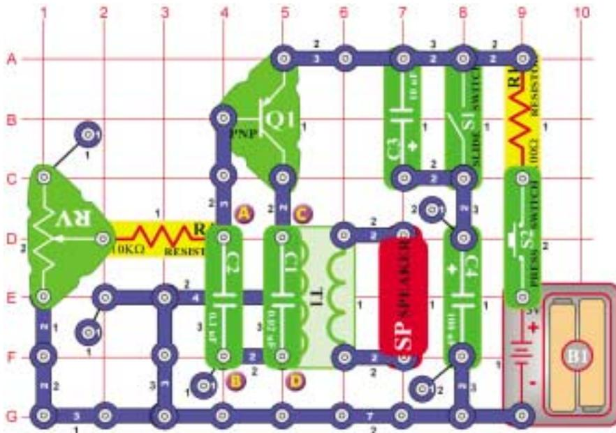
Turn off the switch (S1) and then press and release the switch (S2). You hear a "cat's meow" from the speaker (SP). Now turn the switch (S1) on and the sound is lower and lasts longer. Adjust variable resistor (RV) while the sound is fading away.
