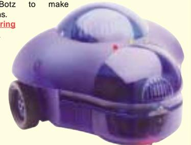
**Movement:** Two (2) wheels driven by two (2) DC motors.
