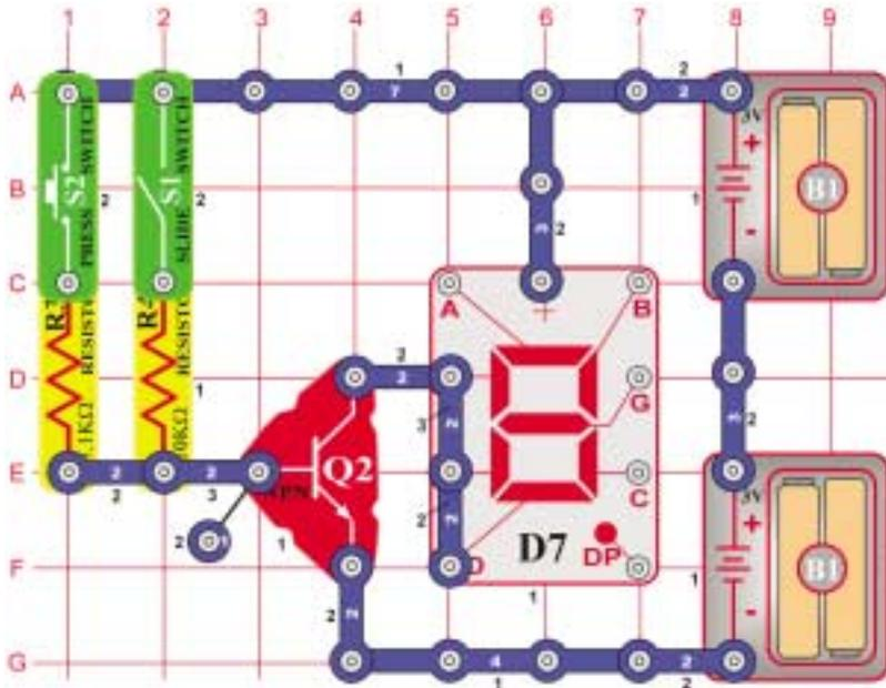
The NOR gate works the opposite of the OR. Using the chart set the switches to the different states. The display lights the letter "L" when either switch is turned on.
