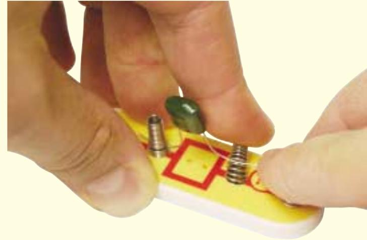
Any component with two wires coming from it (called leads) can be connected with the two-spring socket (?1), assuming the leads are long enough. Usually you will connect different values of resistors or capacitors, but other components like LEDs, diodes, or coils/inductors can also be used. You can usually find electronic components at any store specializing in electronics.
