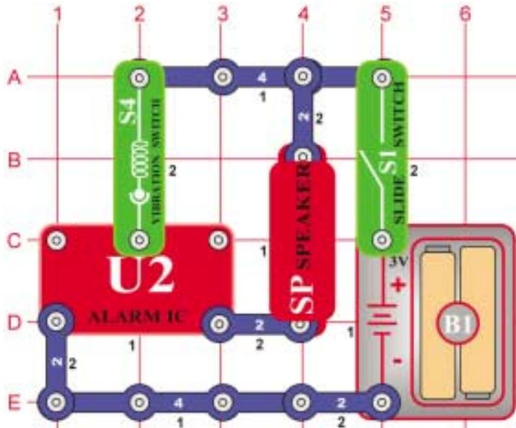
Turn on the slide switch (S1) and shake the circuit or bang on the table, an alarm will sound. Try banging on the table in a regular pattern, and see if you can make the alarm sound continuously.
