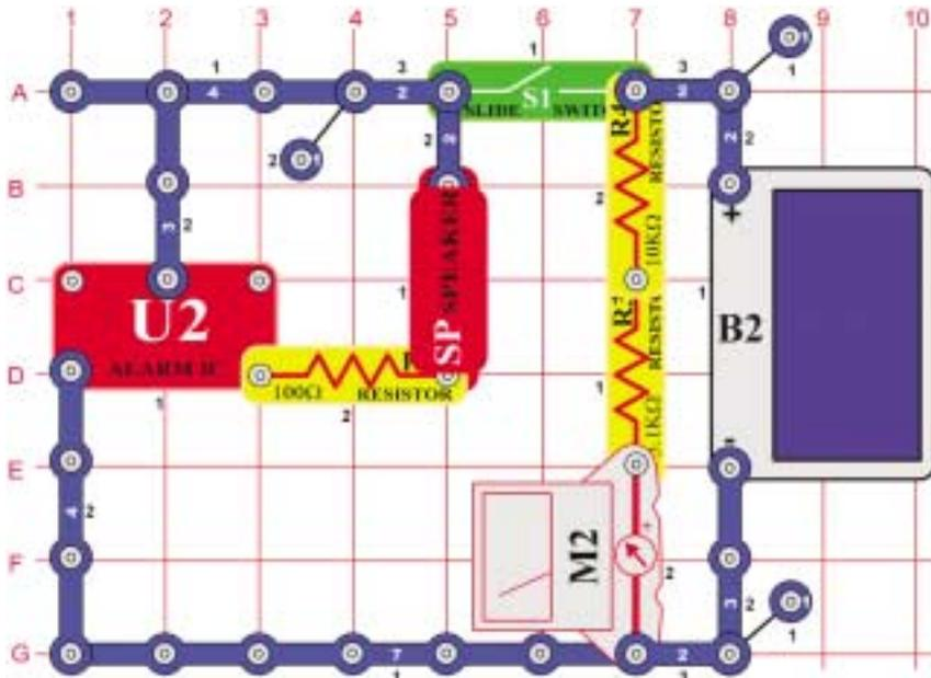
Set the meter (M2) to the 10MA scale. With the slide switch (S1) off, make sure you have a bright light on the solar cell (B2) so the meter reads 10 or higher. Now turn on the switch and listen to the music.
