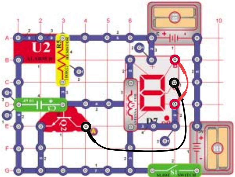
The circuit switches between numbers "9" and "0" on the display. Place a jumper from point A to segment G and point B to segment E.
