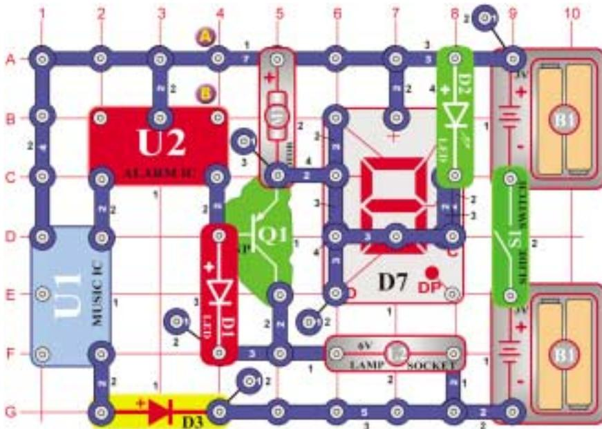
Turn the switch (S1) on. As the output from the IC (U2) drives the transistor (Q1), the motor (M1) spins and the display (D7) lights the letter "S". Instead of turning off as in project #653, the motor slows down and the red LED (D1) lights.
