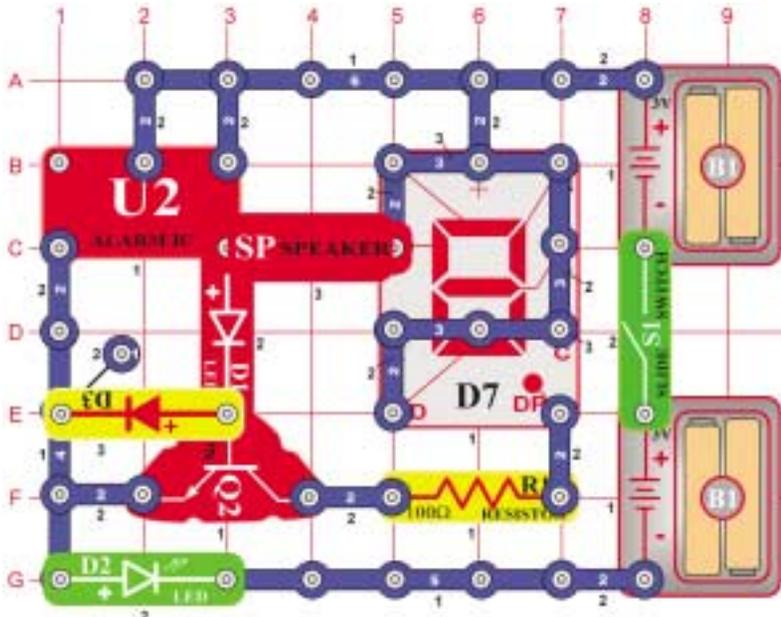
As in project #650, we use the alarm IC (U2) to flash segments and LEDs. Turn the switch (S1) on and the number "0" and green LED (D2) flash as the speaker (SP) sounds. When they turn off, the DP segment lights.
