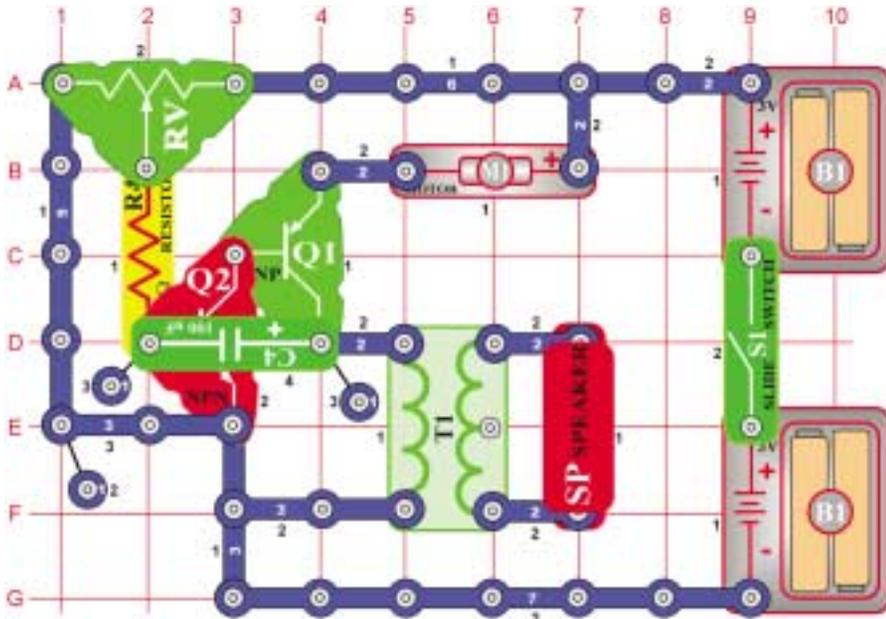
Adjust the variable resistor (RV) to the middle position and turn on the switch (S1). As the circuit oscillates, the motor (M1) moves a short distance as the speaker (SP) sounds. Adjust the variable resistor to different positions seeing how it affects the motor and speaker.
