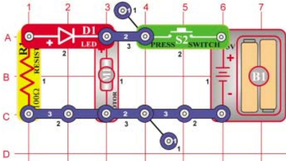
Place the fan on the motor (M1). Hold down the press switch (S2) for a few seconds and then watch the LED (D1) as you release the switch. The LED lights briefly but only after the batteries (B1) are disconnected from the circuit.
