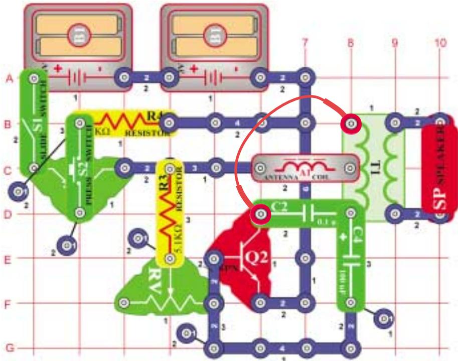
Build the circuit, turn on the switch (S1), and then press switch (S2). Move the control lever of the variable resistor (RV) to change the tone.
