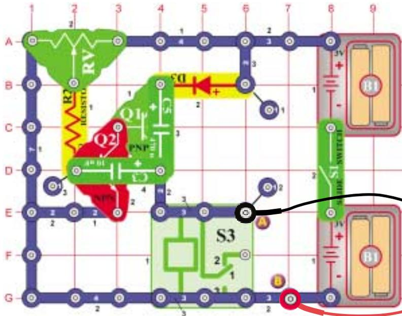
Take a paperclip and straighten it out, bend it in half, and place it into the electromagnet (M3) center. Connect the electromagnet to points A and B with the jumper wires and hold it about 1 inch above the table. Slide the variable resistor (RV) control lever around slowly, you will hear a clicking sound from the relay.
