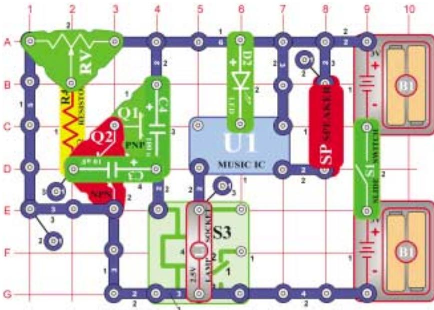
Set the variable resistor (RV) to the far left position and turn the switch (S1) on. The relay's (S3) contacts open and close shorting U1 to ground, causing the sound level to change.
