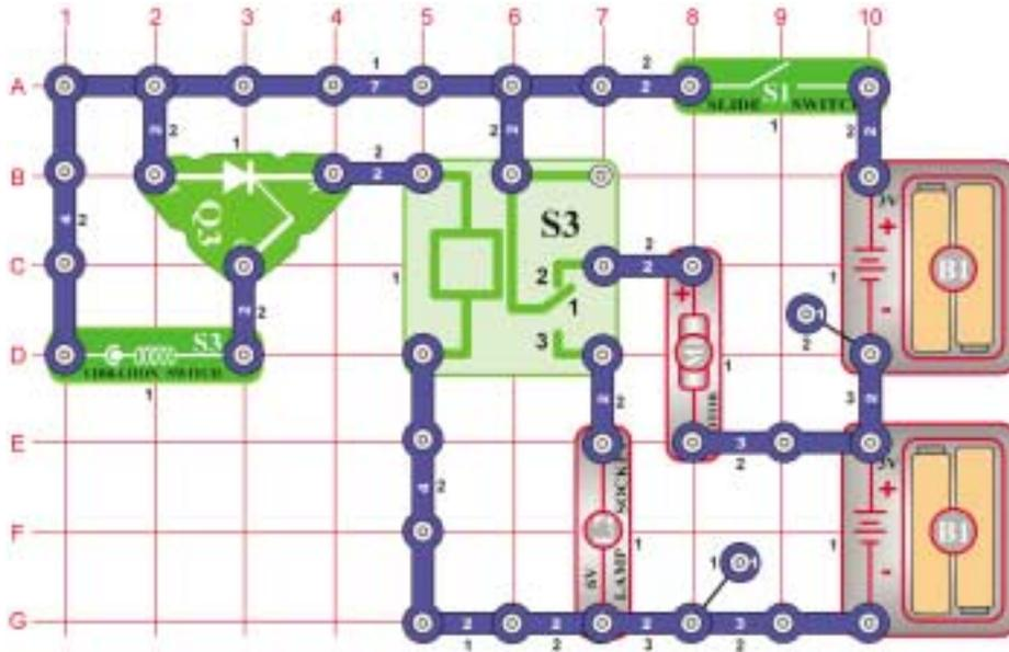
The vibration switch triggers the SCR connecting the relay's coil to the battery. The relay's contacts switch, turning the motor off, and lighting the bulb. The bulb will stay lit until switch S1 is turned off.
