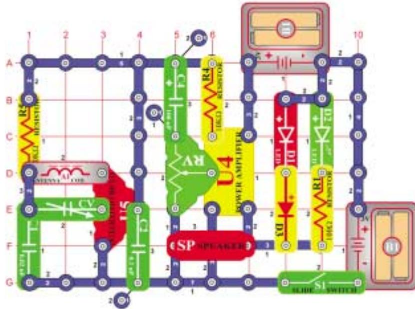
Set the variable resistor (RV) to the middle position and turn the switch (S1) on. Tune the radio by adjusting the variable capacitor (CV). The LEDs (D1 and D2) flicker as the sound is heard.
