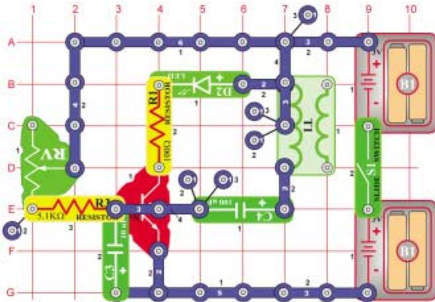
This is an example of how a large strobe light works. Turn the switch (S1) on and the LED (D2) flashes at a certain frequency. Adjust the frequency by adjusting the variable resistor (RV). Now add sound by replacing the 100Ω resistor (R1) with the speaker (SP). Each time the LED lights, the speaker sounds.
