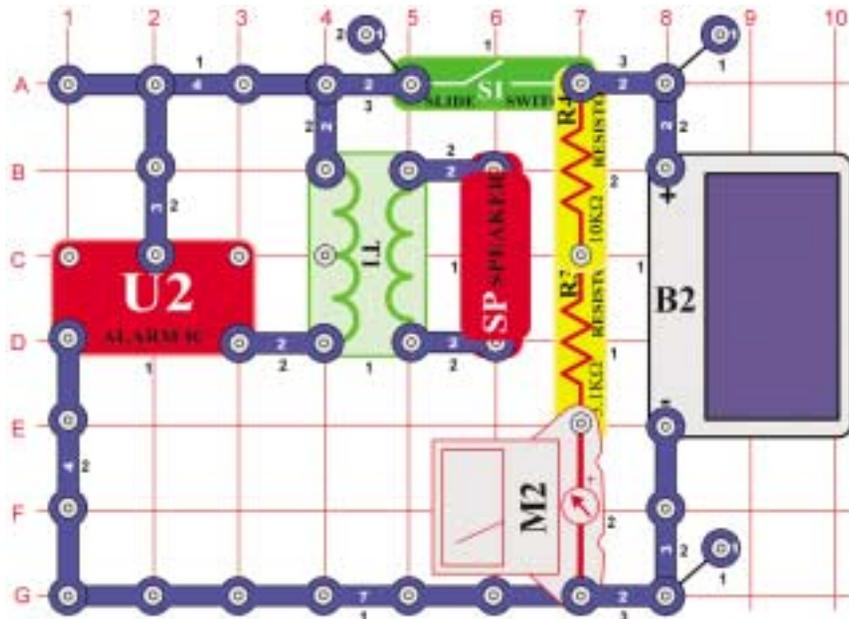
Set the meter (M2) to the 10MA scale. With the slide switch (S1) off, make sure you have enough light on the solar cell (B2) for the meter to read 8 or higher. Now turn on the switch and listen to the music.
