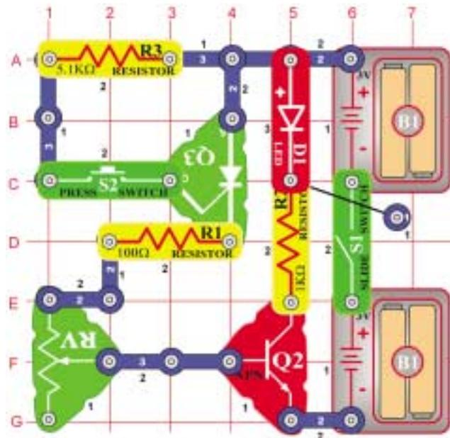
In this circuit the press switch (S2) controls an SCR (Q3), which controls a transistor (Q2), which controls an LED (D1). Set the variable resistor (RV) control lever to the top (toward the press switch).
