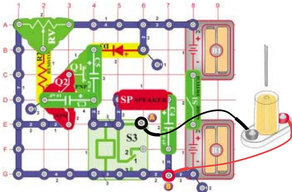
Take a paperclip and straighten it out, bend it in half, and place it into the electromagnet (M3) center. Connect the electromagnet to points A and B with the jumper wires and hold it about 1 inch above the table. Slide the variable resistor (RV) control lever around slowly, you will hear a clicking sound from the relay and speaker.
