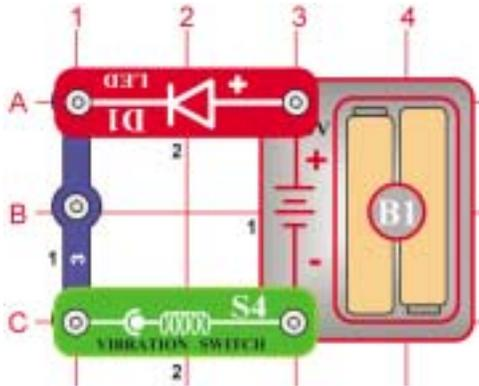
The vibration switch contains two separate contacts; a spring is connected to one of the contacts. A vibration causes the spring to move briefly shorting the two contacts. This simple circuit demonstrates how the vibration switch works. Build the circuit and the LED does not light. Tap the vibration switch or table and the LED lights for every tap. It acts like a temporary switch connecting the battery to the LED.
