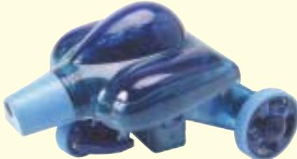
**Movement:** Three (3) wheels driven by a DC motor.
