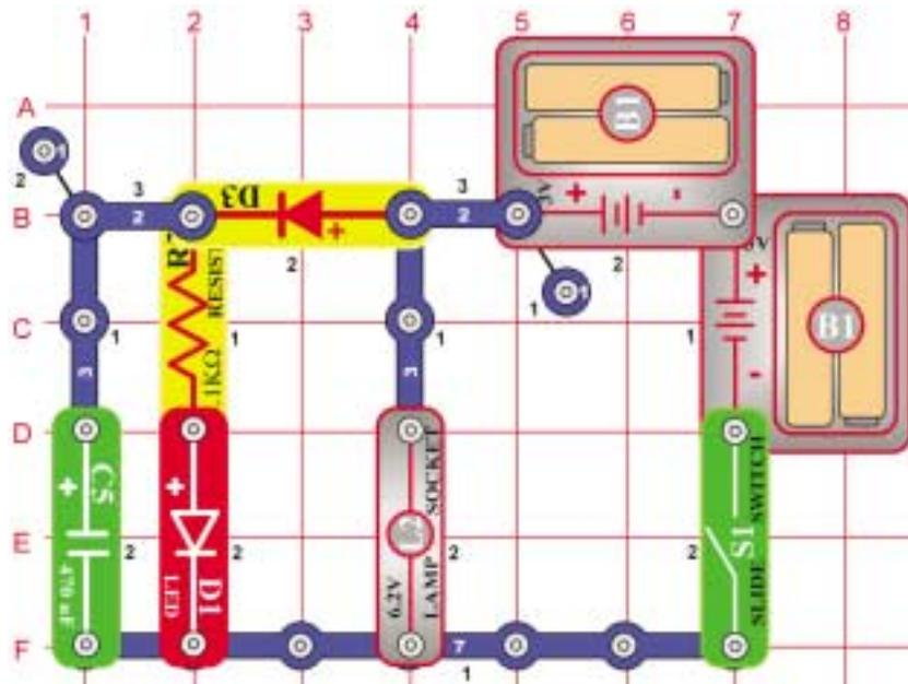
Turn on the switch (S1), the lamp (L2) will be bright and the LED (D1) will be lit. The diode (D3) allows the batteries to charge up capacitor C5 and light the LED.
