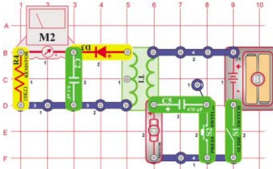
Set the meter (M2) to the 10MA scale. Place the fan on the motor (M1) and turn on the switch (S1), the meter measures the current on the other side of the transformer (T1).
