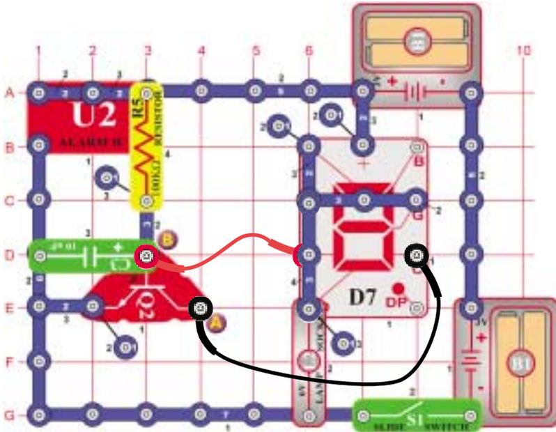
The circuit switches between numbers "2" and "3" on the display. Place jumpers from point A to segment C and point B to segment E.
