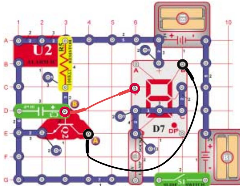
The circuit switches between letters "b" and "d" on the display. Place a jumper from point A to segment B and point B to segment F.
