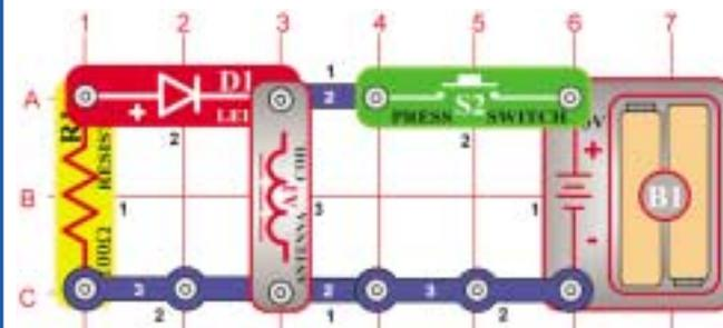
Hold down the press switch (S2) and then watch the LED (D1) as you release the switch. The LED lights briefly but only after the batteries (B2) are disconnected from the circuit.
