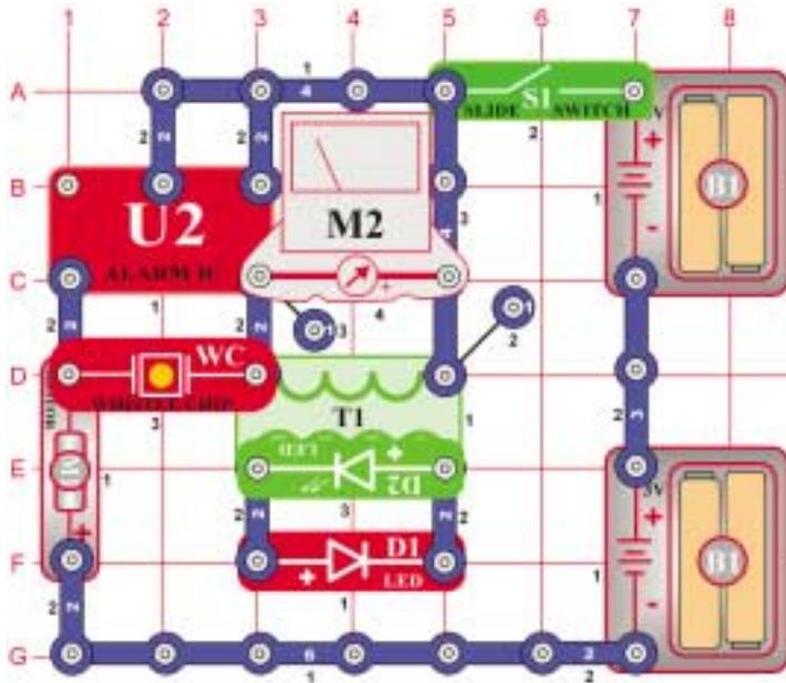
Turn on the switch (S1) and now you have a pulsing motor and LEDs circuit. Replace the meter (M2) with the 470 $\mu$ F capacitor (C5) to change the rate the LEDs (D1 and D2) flash.
