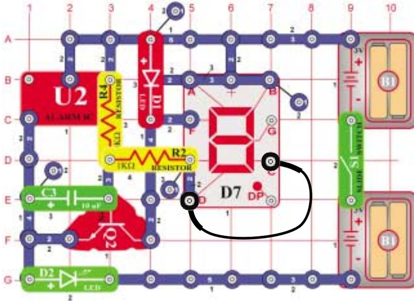
Turn the switch (S1) on, segments A, B, and F light and then segments C, D, and E. The two groups of segments are connected to different voltages. As the voltage changes from high to low, the segments toggle back and forth.
