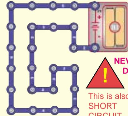
When the switch (S1) is turned on, this large circuit has a **SHORT CIRCUIT** path (as shown by the arrows). The short circuit prevents any other portions of the circuit from ever working.
