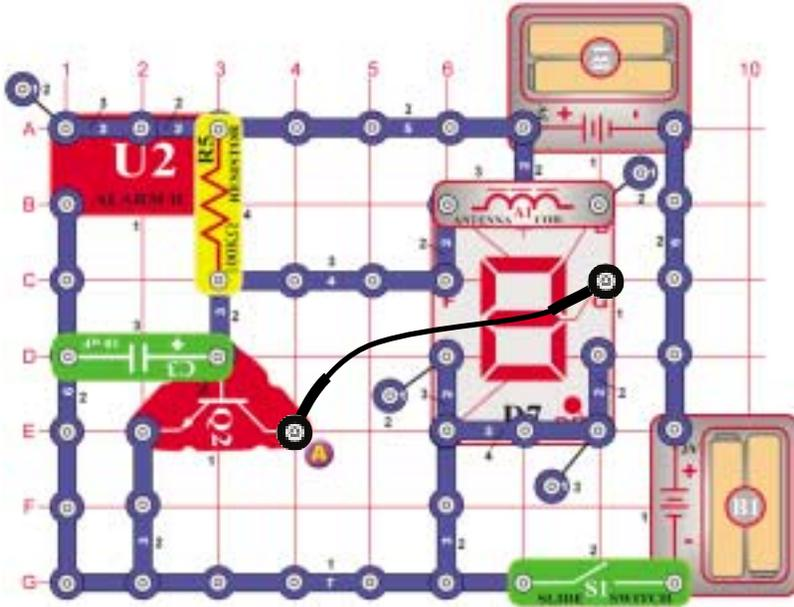
The circuit switches between upper case "O" and lower case "o". Place a jumper from point A to segment G. The DP segment will also light.
