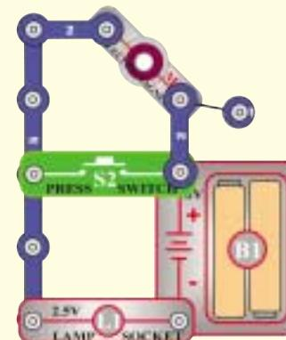
31. **Vibration Switch (S4):** Build the mini-circuit shown here and shake the base grid. The LED should go on and off as you shake.
