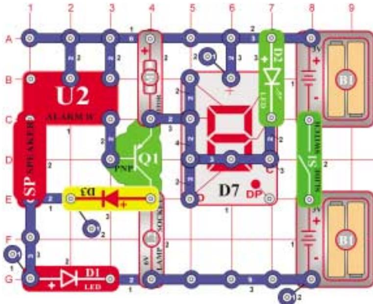
Turn the switch (S1) on and the speaker (SP) outputs the sounds from the alarm IC (U2). The IC also drives the transistor (Q1) causing the motor (M1) to spin and lights to flash.
