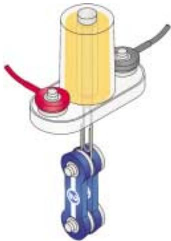
Snap two 2-snaps around a paperclip and lift them with the electromagnet, as shown here on the left.
