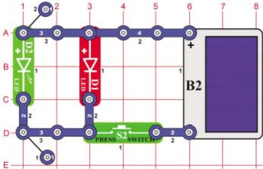
Place this circuit near different types of lights and press the switch (S2), if the light is bright enough then the LEDs (D1 and D2) will be lit. Find out what types of light sources make it brightest.
