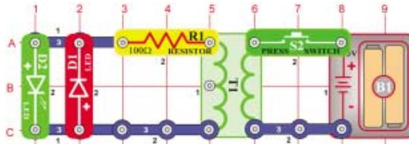
Watch the LEDs (D1 and D2) as you press or release the switch (S2). The red LED (D1) lights briefly just as you press the switch and the green LED (D2) lights briefly just after you release it, but neither lights while you hold the switch down. Why?
