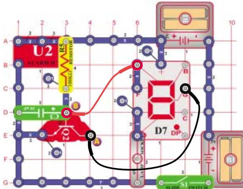
The circuit switches between letters "c" and "C" on the display. Place a jumper from point A to segment G and point B to segment A.
