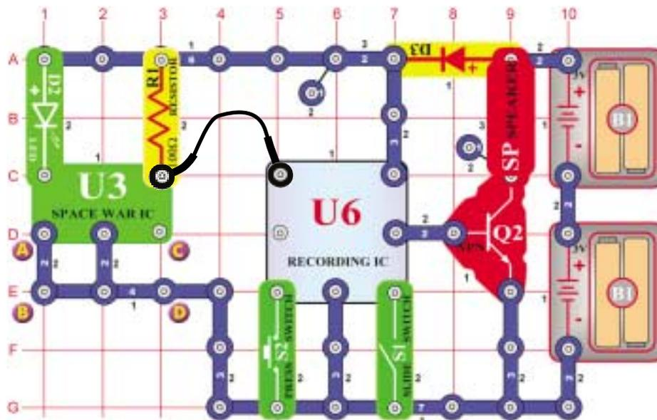
The circuit records the sounds from the space war IC (U3) into the recording IC (U6). Turn on the switch (S1) and the first beep indicates that the IC has begun recording. When you hear two beeps, the recording has stopped. Turn off the switch (S1) and press the switch (S2). You will hear the recording of the space war IC before each song is played.
