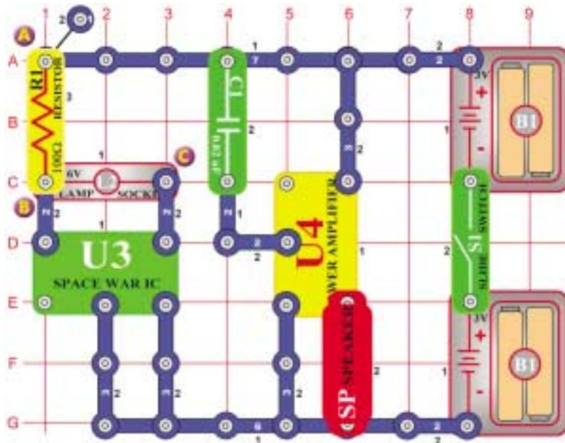
Turn the switch (S1) on and you should hear a tone from the speaker (SP). Connect the jumper wire from A to B, the lamp (L2) lights and the tone changes. Move the jumper wire from B to C to hear an assortment of sounds.
