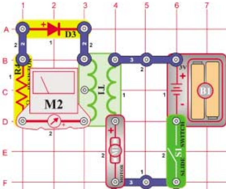
By placing the meter (M2), diode (D3) and current limiting resistor (R4) on the transformer (T1), you can measure the current. Turn on the slide switch (S1) and the motor (M1) starts spinning. Current flows through the primary and secondary of the transformer.
