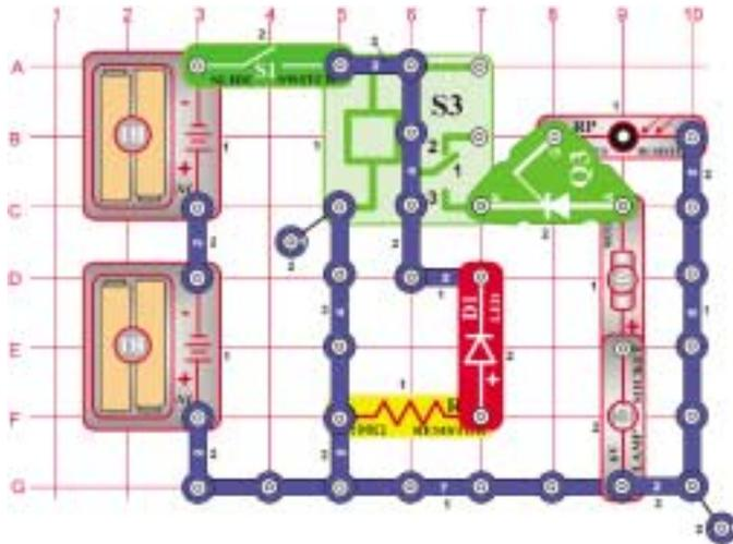
Cover the photo resistor (RP) with your finger. Turn on the switch (S1), and only the LED (D1) lights. The relay (S3) connects the motor (M1) and the bulb (L2) to the batteries, but the motor and bulb are powerless until a voltage is applied to the SCR's gate.
