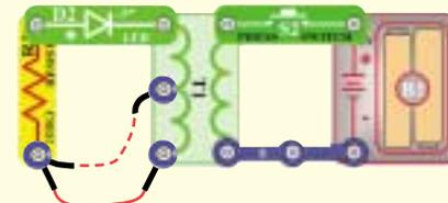
26. **Diode (D3):** Build the mini-circuit shown here, the LED should light. Reverse the direction of D3, the LED should not light now.
