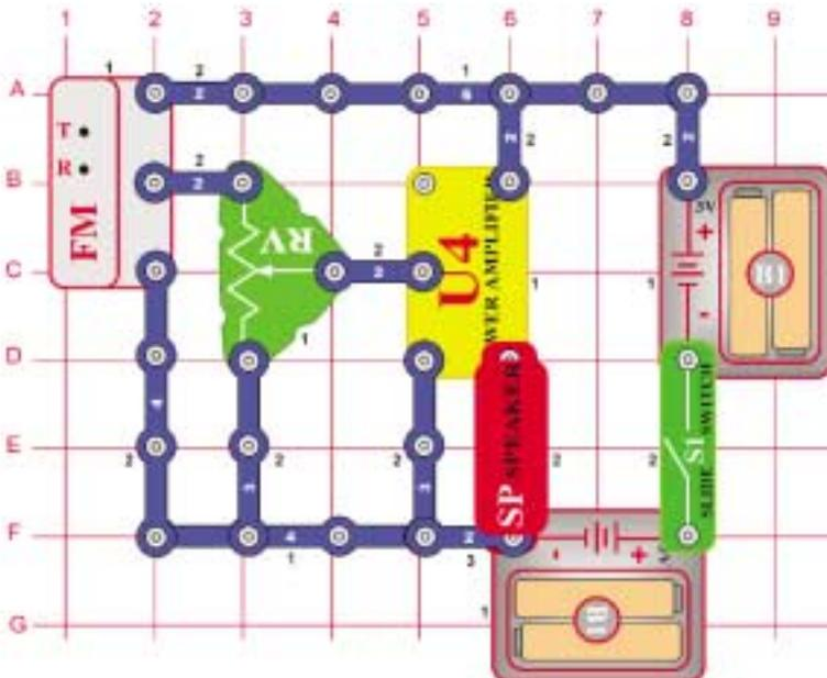
Turn on the switch (S1) and press the R and then the T button. When a station is heard, adjust the volume using the variable resistor (RV). The resistor controls the amount of signal into the power amp.
