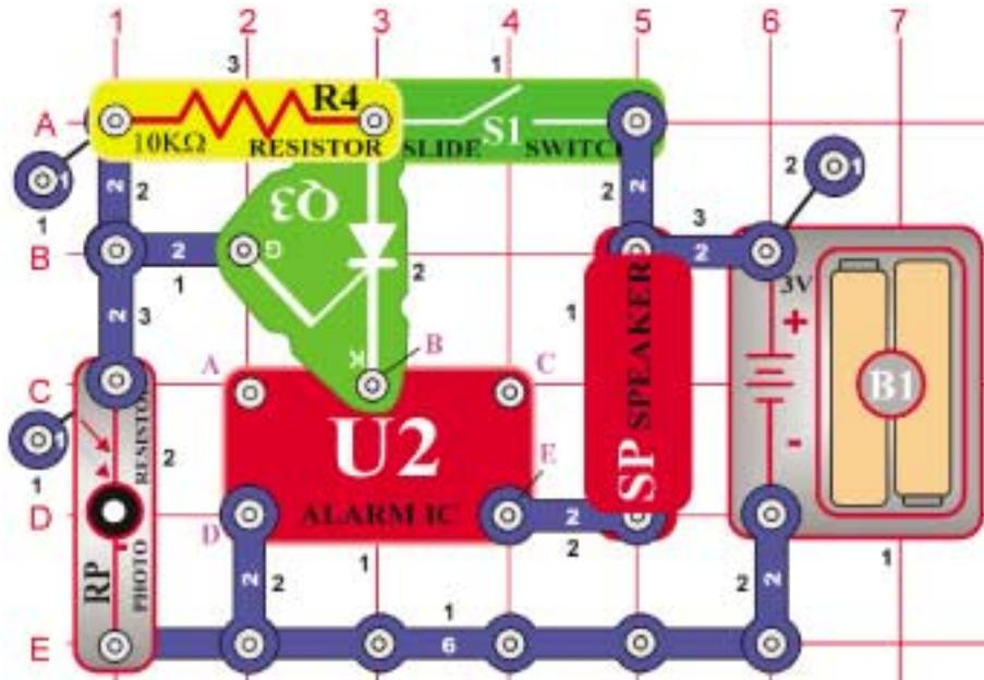
As the photo resistor (RP) is exposed to light, its resistance is very low, thereby connecting the gate of the SCR (Q3) to ground. This prevents the SCR from conducting, connecting the alarm IC (U2) to the batteries. The alarm IC remains off until the light is blocked, triggering the SCR.
