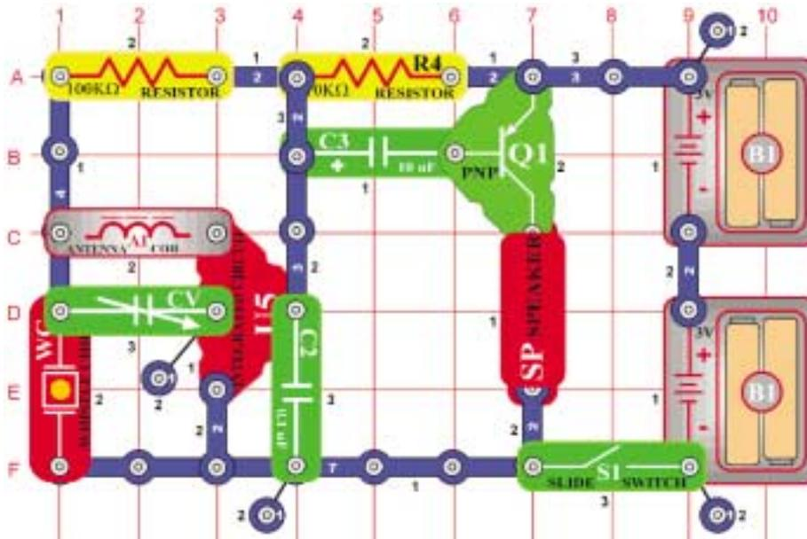
Turn on the slide switch (S1) and adjust the variable capacitor (CV) for a radio station.
