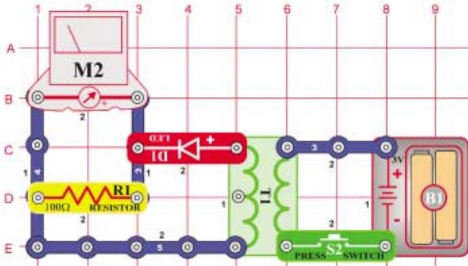
Pressing and releasing the press switch (S2) continuously generates an AC current. The LED (D1) is used to convert the AC current to DC current because it only allows the current to flow in one direction. The LED should light as the meter (M2) deflects to the right only. Without the LED, the meter would deflect in both directions.
