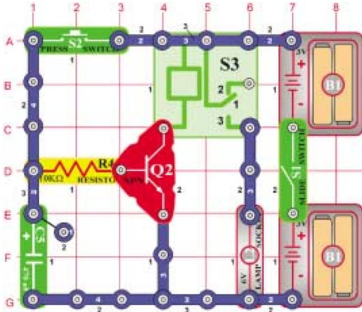
The transistor (Q2) acts as a switch, connecting the relay (S3) to the batteries. As long as there is positive voltage on the transistor's base, the bulb (L2) will light.
