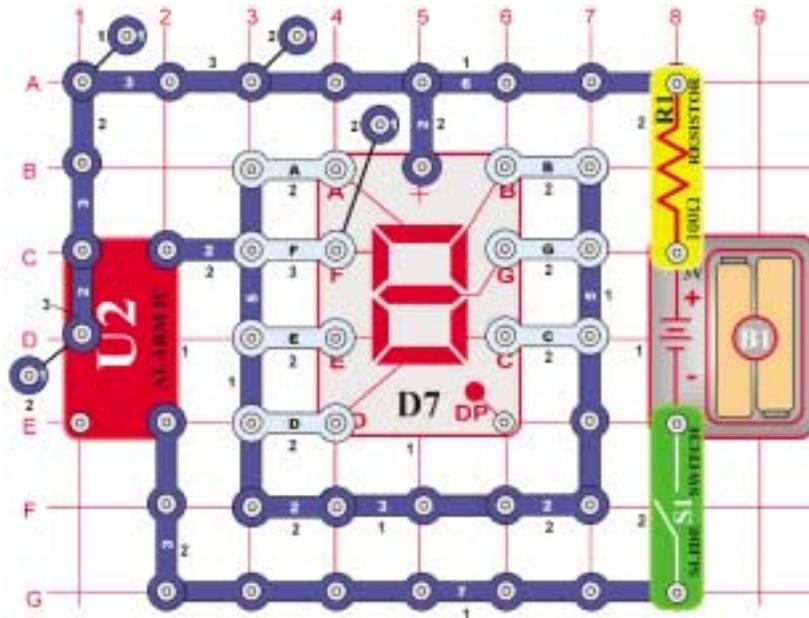
**OBJECTIVE:** Use the Alarm IC as a switch to flash the letters "C & E".
