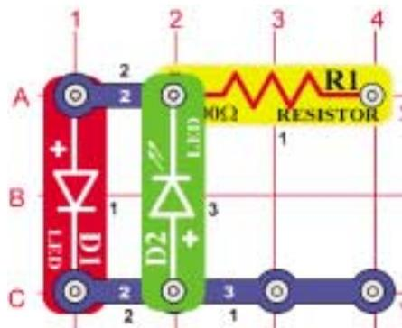
Use this circuit to check the polarity of a battery. Connect your battery to X and Y on the drawing using the jumper cables (your 3V battery pack (B1) can also be snapped on directly instead). If the positive (+) side of your battery is connected to X, then the red LED will be on, if the negative (-) side is connected to X then the green diode will be on.
