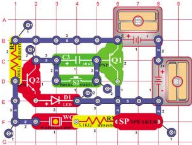
Build the circuit shown and press the press switch (S2). The circuit starts to oscillate. This generates the sound of a high pitch bell.
