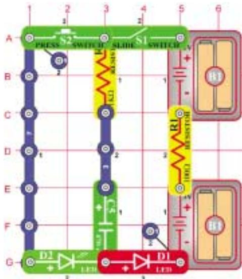
Turn on the slide switch (S1) for a few seconds, then turn it off. The red light emitting diode (LED, D1) is initially bright but goes dim as the batteries charge up the capacitor (C5). The capacitor is storing electrical charge.
