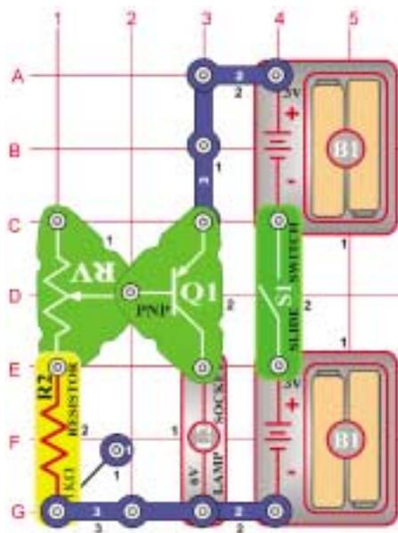
**OBJECTIVE:** *To demonstrate adjusting the gain of a transistor*
