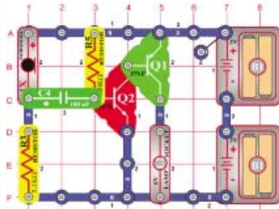
Install the parts. The lamp (L1) will be on. It will be off as long as you blow on the mic (X1). Speaking loud into the mic will change the brightness of the lamp.
