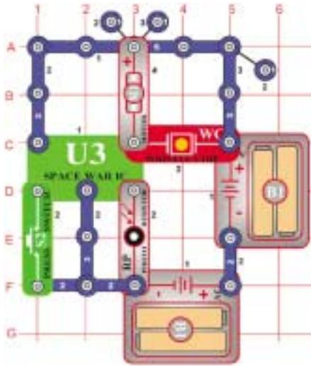
Place the fan onto the motor. Space war sounds are heard if light shines on the photosensitive resistor OR if you press the press switch (S2), the fan may start to spin, but will only get to high speed if you do BOTH. Try various combinations of shining light and holding down the press switch.
