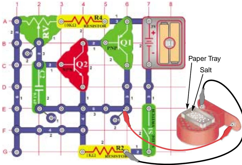
Build the circuit shown on the left and connect the speaker using the two (2) jumper wires. Then, lay the speaker on a flat hard surface.
