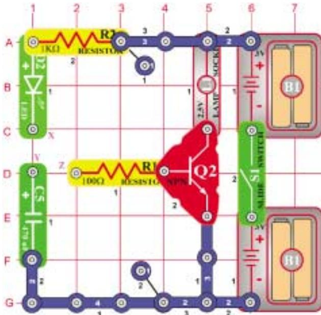
Put on the switch, then connect points X and Y (use a 2-snap wire). The green LED will flash and then go out, as the 470µF capacitor is charged with electricity. Now disconnect X and Y and instead make a connection between Y and Z. The 6V bulb will flash as the electricity stored in the 470µF discharges through the resistor and transistor. The capacitor was storing electricity to be used at a later time, just like a battery does!
