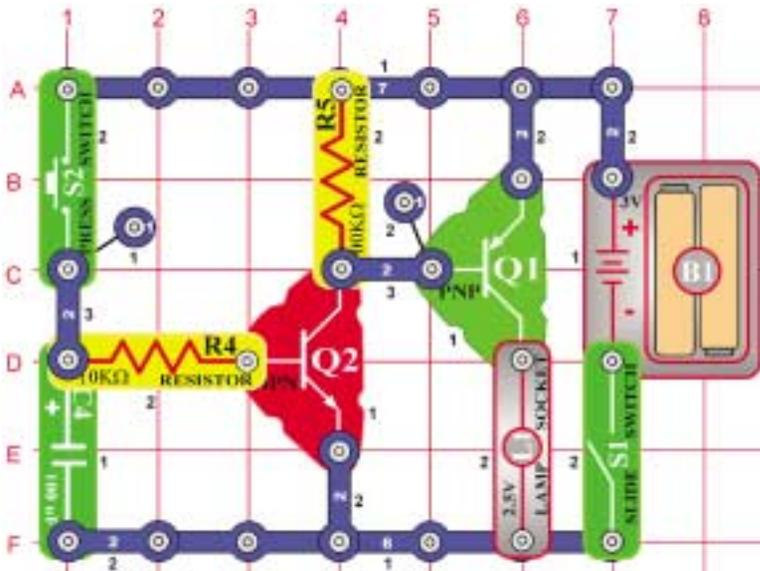
Turn on the switch and press the press switch (S2). The lamp stays on for a few seconds after you release the press switch.
