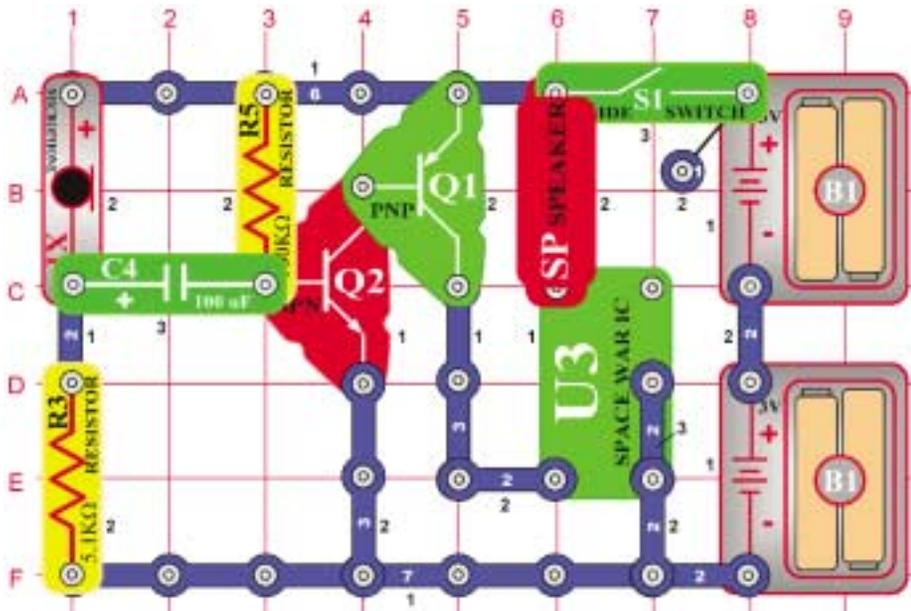
Build the circuit and turn it on, you hear a space war. Since it is loud and annoying, try to shut it off by blowing into the microphone (X1). Blowing hard into the microphone stops the sound, and then it starts again.
