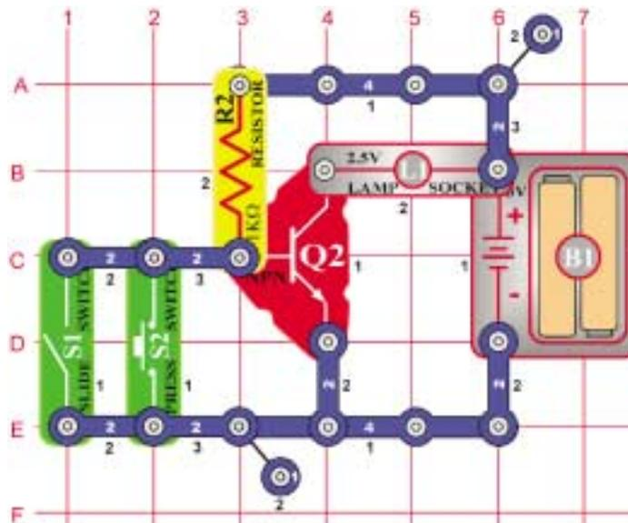
Build the circuit on the left. You will find that the lamp is on when neither the slide switch (S1) NOR the press switch (S2) are on. This is referred to as an NOR gate in electronics and is important in computer logic.
