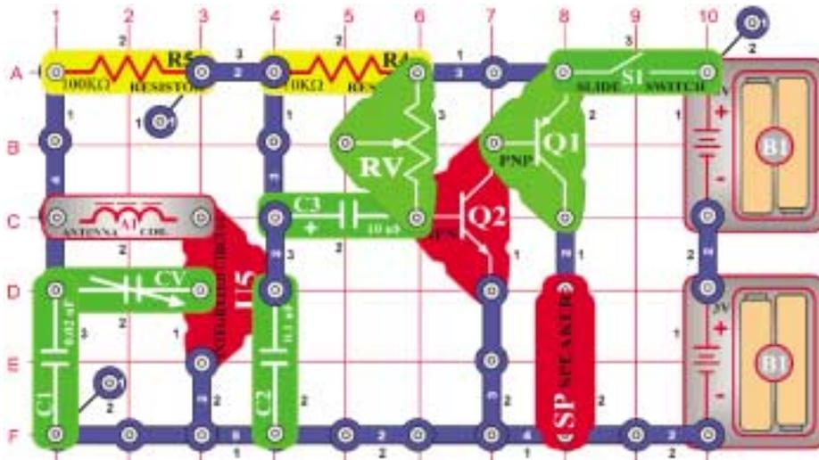
When you close the slide switch (S1), the integrated circuit (U5) should amplify and detect the AM radio waves. Tune the capacitor (CV) to the desirable station. The adjustable resistor (RV) is used as a simple resistor since the center tap is not used. The two transistors drive the speaker to complete the radio. The radio will not be very loud.
