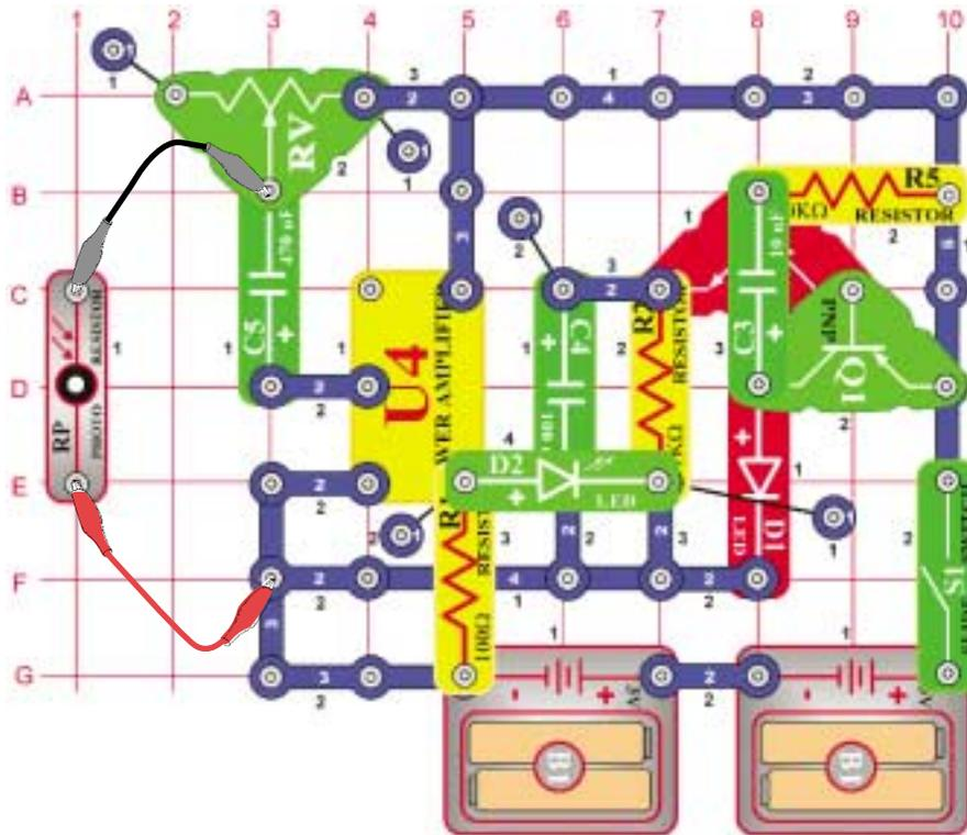
Connect two jumper wires to the photosensitive resistor (RP) as shown. Set the adjustable resistor (RV) control to the far-left side. Turn the switch on and the red LED starts flashing. Hold the photosensitive resistor over the red LED so it is facing it. As the red LED lights, so will the green. This is an example of an optocoupler/opto-isolator. An electric device that transmits signals without an electrical connection between the light source (input) and the light detector (output).
