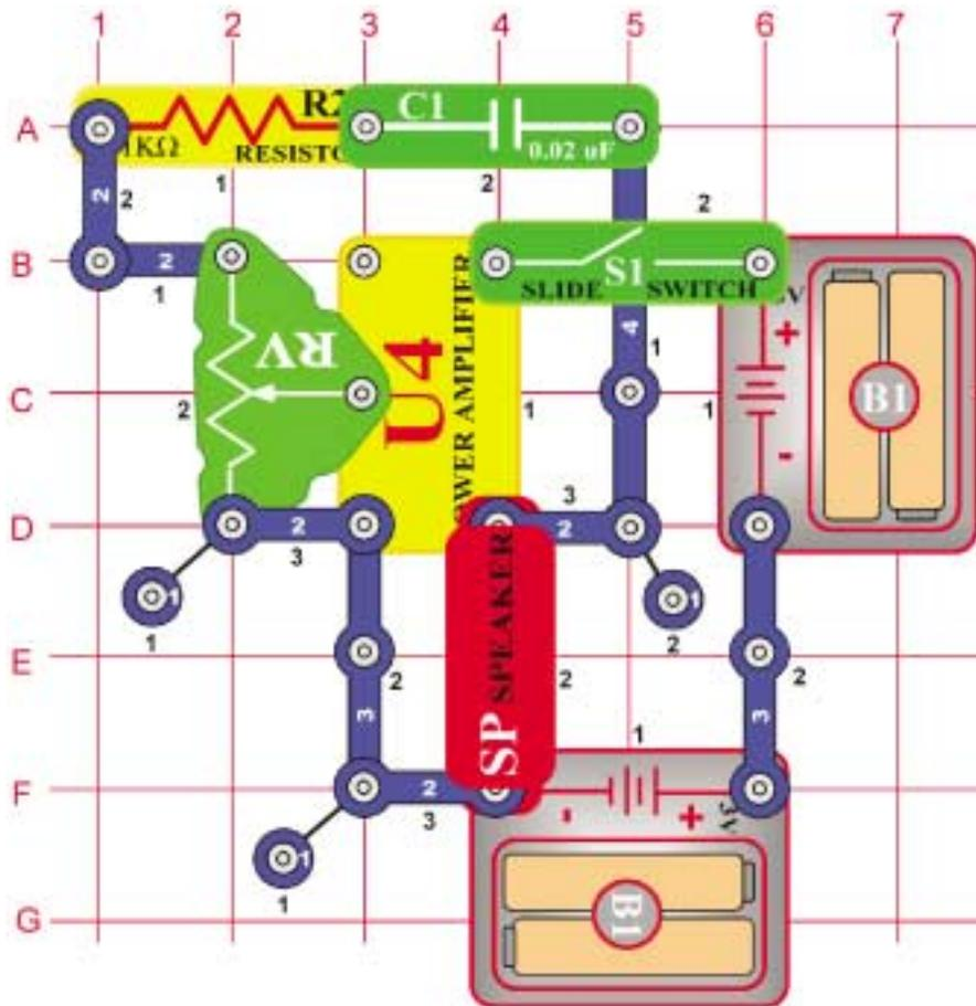
When you turn on the slide switch (S1) the trombone should start playing. To change the pitch of the note, simply slide the adjustable resistor control (RV) back and forth. By turning the slide switch (S1) on and off and moving the slider, you will be able to play a song much like a trombone player makes music. The switch represents air going through the trombone, and the control is same as trombone slider bar. The circuit may be silent at some positions of the resistor control.
