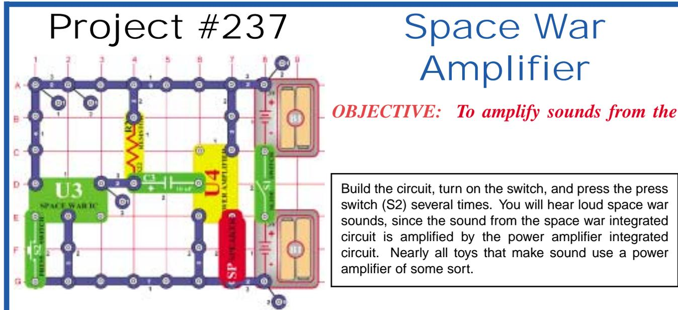
Build the circuit, turn on the switch, and press the press switch (S2) several times. You will hear loud space war sounds, since the sound from the space war integrated circuit is amplified by the power amplifier integrated circuit. Nearly all toys that make sound use a power amplifier of some sort.
