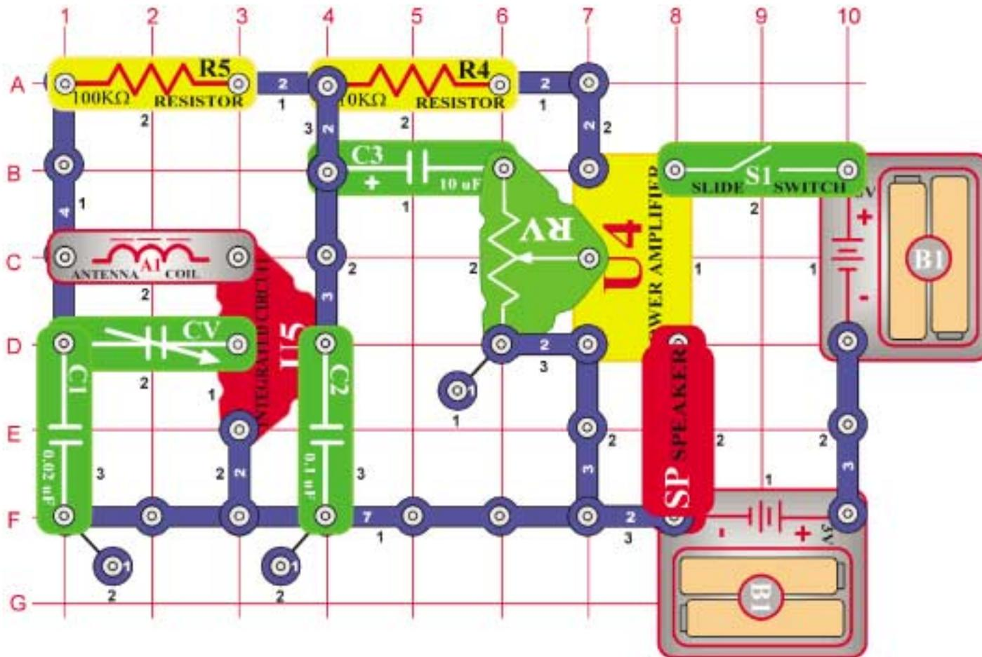
When you close the slide switch (S1), the integrated circuit (U5) should amplify and detect the AM radio waves all around you. The variable capacitor (VC) can be tuned to the desirable station. Varying the adjustable resistor (RV) will make the audio louder or softer. The power amplifier (U4) drives the speaker (SP) to complete the AM radio project.
