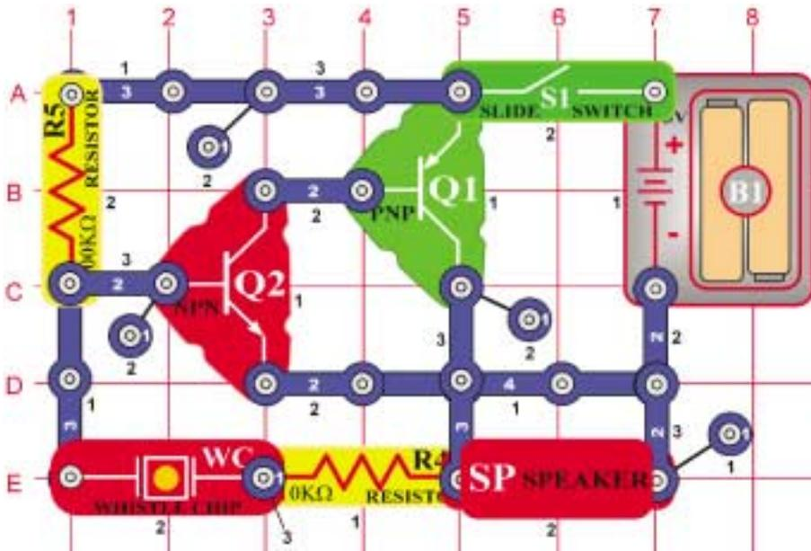
Build the circuit, as the name suggests this circuit is similar to that in Project 206. Turn it on, you hear a middle-frequency sound.
