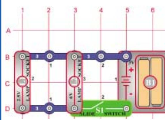
Turn on the slide switch (S1) and both lamps will light. If one of the bulbs is broken then the other will still be on, because the lamps are in parallel. An example of this is most of the lights in your house; if a bulb is broken on one lamp then the other lamps are not affected.
