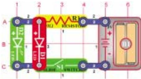
Put on the switch and both LEDs will be on and equally bright. This is because the diodes are in *parallel*, and the electric current divides equally between them.
