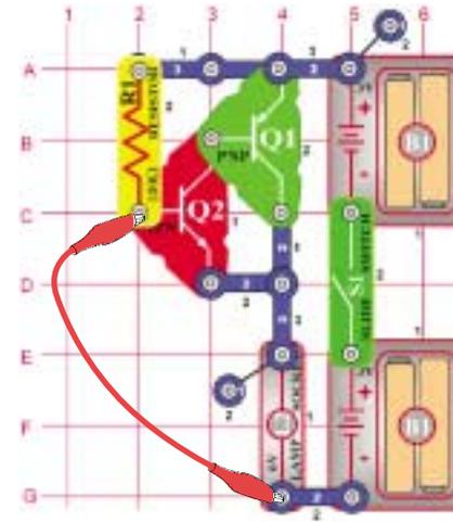
This light alarm circuit uses two (2) transistors and both sets of batteries. Build the circuit with the jumper connected as shown, and turn it on. Nothing happens. Break the jumper connection and the light turns on. You could replace the jumper with a longer wire and run it across a doorway to signal an alarm when someone enters.
