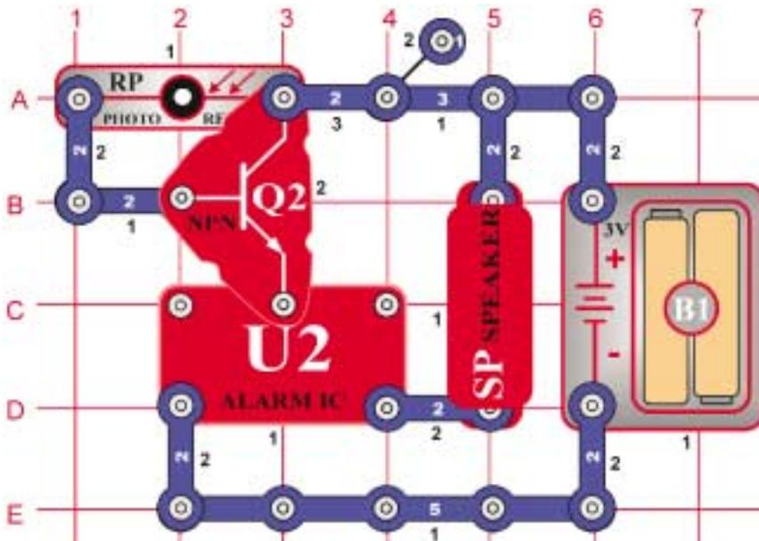
The alarm will sound, as long as light is present. Slowly cover the photosensitive resistor (RP), and the volume goes down. If you turn off the lights, the alarm will stop. The amount of light changes the resistance of the photosensitive resistor (less light means more resistance). The photosensitive resistor and transistor (Q2) act like a dimmer switch, adjusting the voltage applied to the alarm.
