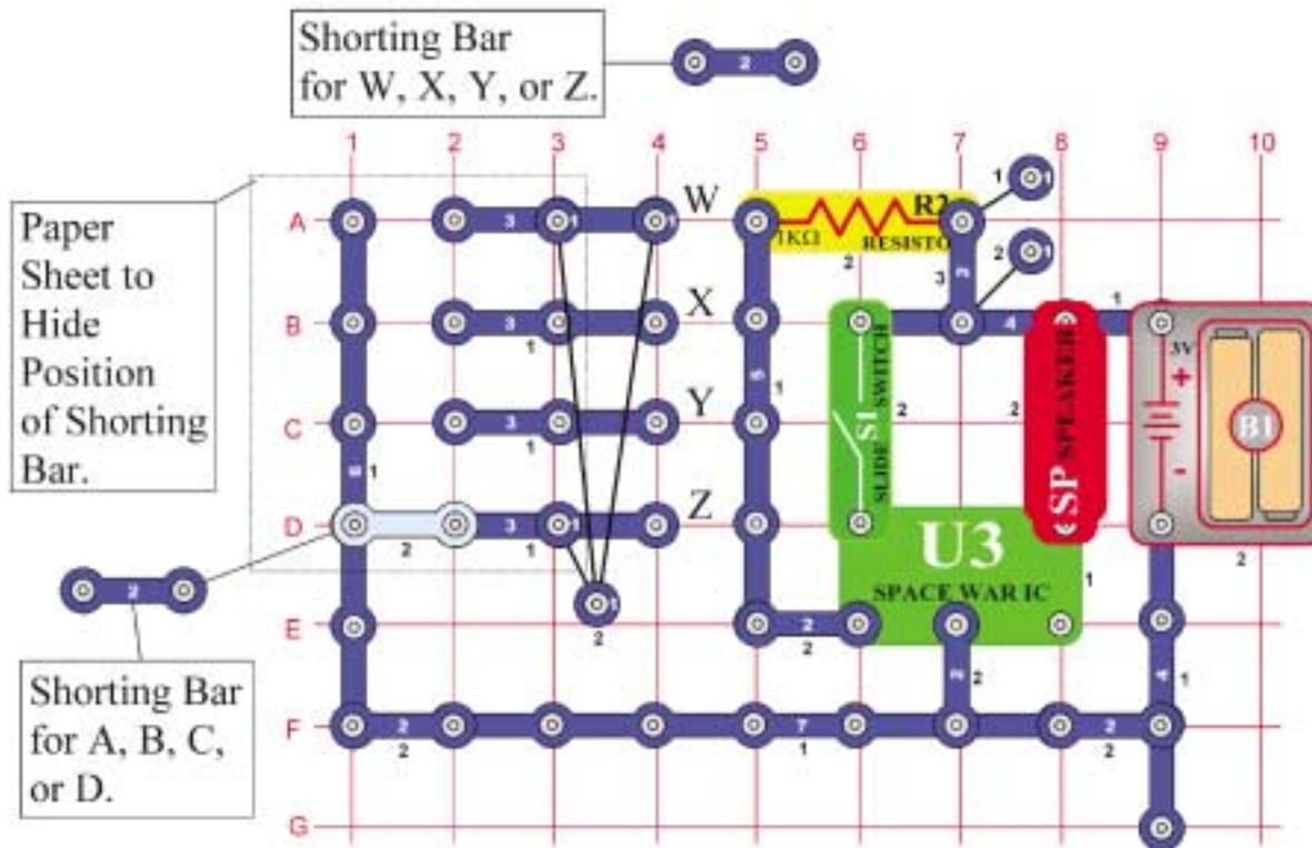
Build the circuit shown on the left. It uses two (2) 2-snap wires as shorting bars.
