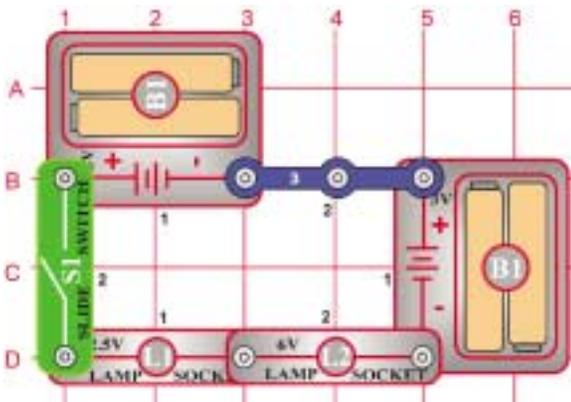
Turn on the slide switch (S1) and both lamps will light. If one of the bulbs is broken then neither will be on, because the lamps are in series. An example of this is the strings of small Christmas lights; if one bulb is damaged then the entire string does not work.
