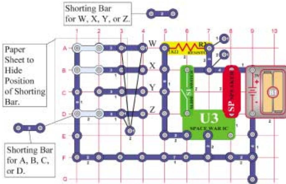
Use the circuit from Project 233, but place three (3) 2-snap wires ("shorting bars") under paper as shown on left.
