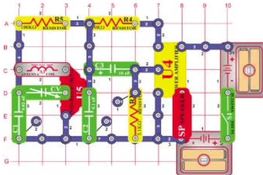
When you close the slide switch (S1), the integrated circuit (U5) should detect and amplify the AM radio waves. The signal is then amplified using the power amplifier (U4), which drives the speaker. Tune the capacitor (CV) to the desirable station.
