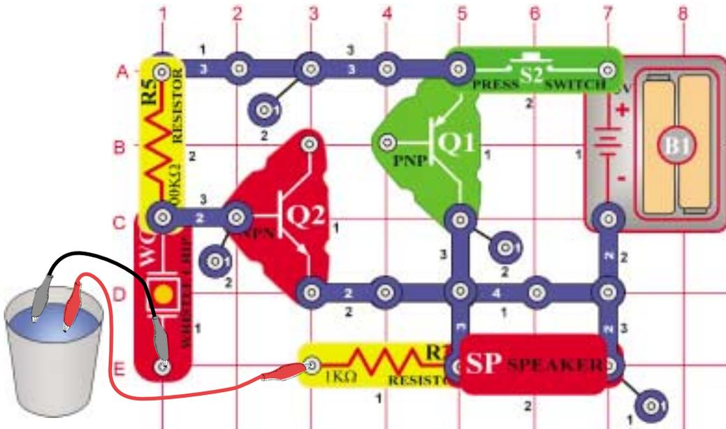
Build the circuit at left and connect the two (2) jumpers to it, place the loose ends of the jumpers into an empty cup (without them touching each other). Press the press switch (S2) - nothing happens. Add some water to the cup and an alarm sound will sound. Add salt to the water and the tone changes.
