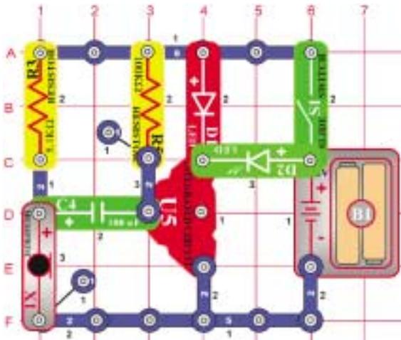
Turn the slide switch (S1) on. There will be only a weak light emitting from the green LED. By blowing on the mic (X1) or putting it near a radio or TV set, the green LED will emit light, and its brightness changes as the loudness changes.
