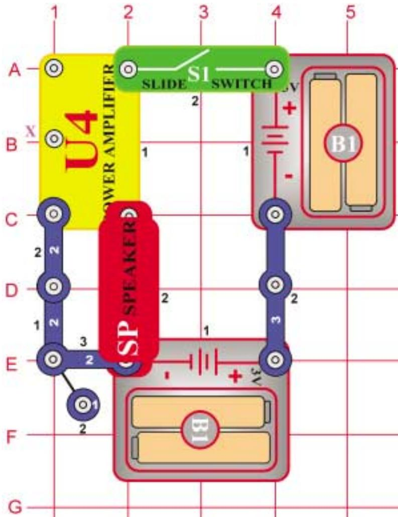
When you turn on the slide switch (S1), the power amplifier should not oscillate. You should be able to touch point X with your finger and hear static. If you do not hear anything, then try touch point X with one of the snaps on any part. High frequency clicks or static should be coming from speaker indicating that the amplifier is powered on and ready to amplify signals.
