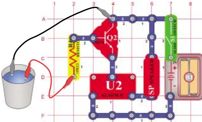
Build the circuit at left and connect the two (2) jumpers to it, place the loose ends of the jumpers into an empty cup (without them touching each other). Turn on the switch - nothing happens. This circuit is designed to detect water and there is none in the cup. Add some water to the cup - an alarm sounds!
